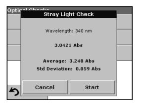
5. The "Average" and "Std Deviation" are calculated from 100 successive absorbance measurements. The result is displayed and is to be compared with the nominal/standard data (given in the quality control certificate) of the sample cuvette/cell.
